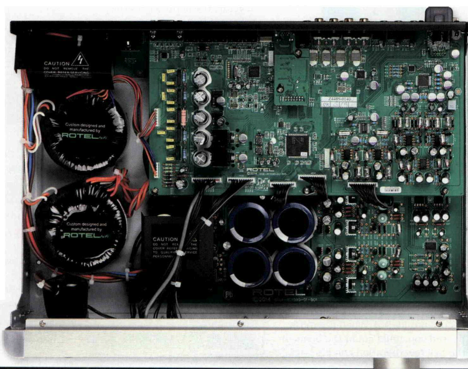
RIGHT: Separate linear PSUs feed the RC-1590's digital and analogue circuits, the former based on an XMOS USB front-end and 32-bit TI DAC (maximum 192kHz/24-bit media supported)
